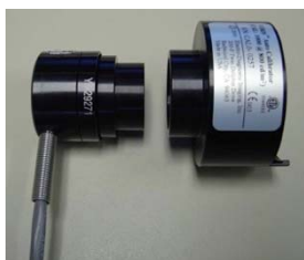
Spot Calibrator with (CA) Adapter
