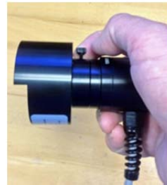
Spot Calibrator with ECCA attached
